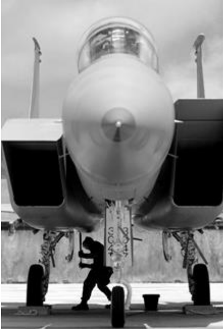
An F-15, formerly the F-X, showing its variable geometry inlets in two positions.
